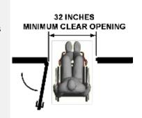
Do the push or pull sides of doors have adequate clearance from the side and front of the doorway to allow customer to reach the handle and maneuver around and through the door opening? See section 404.2.4 of the 2010 ADA Standards for the full requirements.
