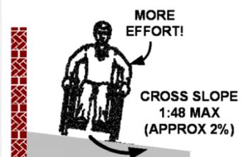
Note: When the running slope along the direction of travel on walking surface is greater than 1:20 (5%) the route is considered a “ramp”. See Items 4-8 on the next two pages.
