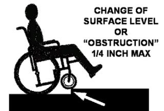
Where vertical changes in surface level are between 1/4 and 1/2 IN in height, is the level change beveled (slope 1:2 or less)?
