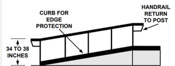
Do handrails continue to extend horizontally at least 12 IN at the top and bottom landings of the ramp and do these extensions return to the wall, floor or post?
