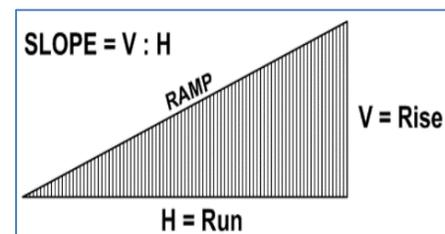
To measure the slope, lay one end of a carpenter's level on the uphill side of the ramp, lift the downhill end of the tool to bring it to level (bubble in the middle), and measure the distance between the downhill bottom edge of the level and the ramp surface. See the figure. In this case the slope is a 3-inch rise over a 36-inch horizontal distance or the ratio of 1:12.
