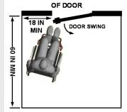
MANEUVERING CLEARANCE AT DOOR FRONT APPROACH TO PUSH FACE OF DOOR WITH A CLOSER AND LATCH
